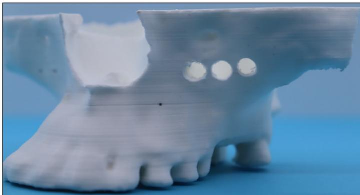
*Figure 22. A printed 3D model with three holes created – medial central and distal*
