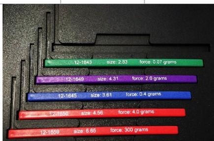
Fig. 2-4 Set of 5 Monofilaments
