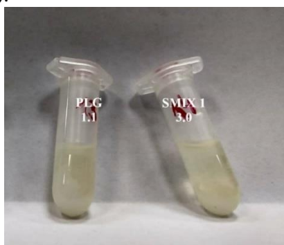
Figure 16: SDEDDS models PLG 1.1 and Smix1 3.0 exhibited phase separation after four cycles of analytical centrifugation.
