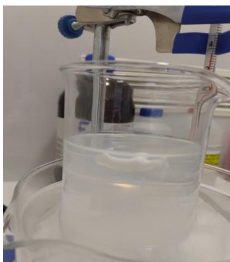
Figure 19: Determination of SET (Self-Emulsification Time)
