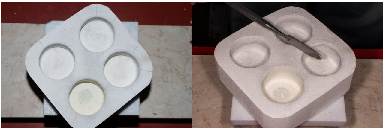
Fig.29. Residual ash content left after burn-out of the four examined specimens.
