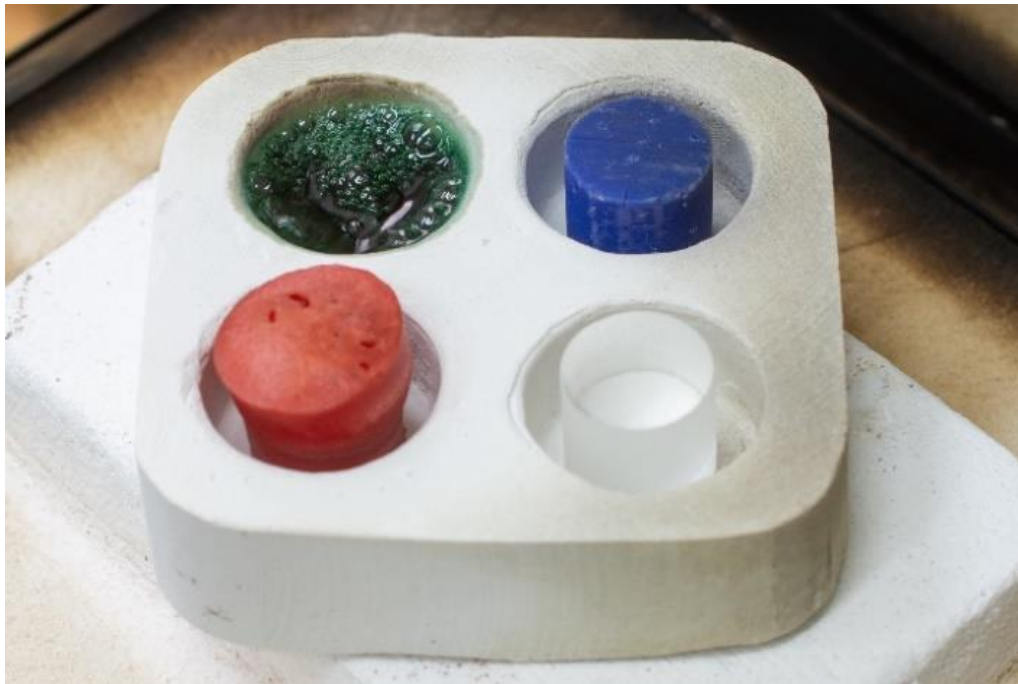
Fig.22 - B. Structural changes of the samples at 250oC, after the 10 min. hold.
