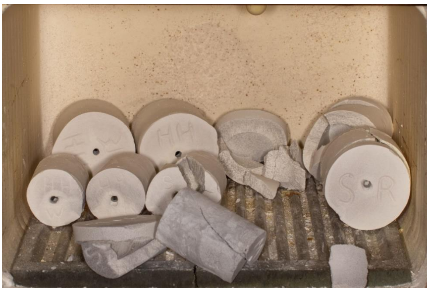
Fig.40. The experimental molds at 980°C.
