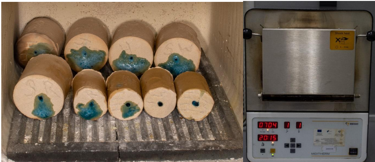
Fig.10. The observed molds made of WiroFine ® and inserted into the furnace at 700°C.
