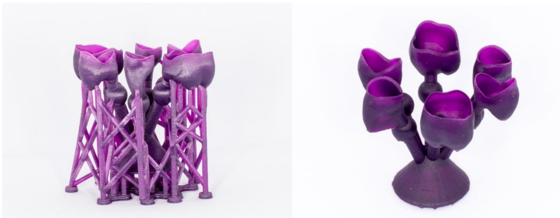
Fig.49. The crown patterns and casting system that are produced by SLP technology. After supporting structures removal, the digitally generated casting cone can be used as a base for mounting of the casting system to the prefabricated casting cone.
