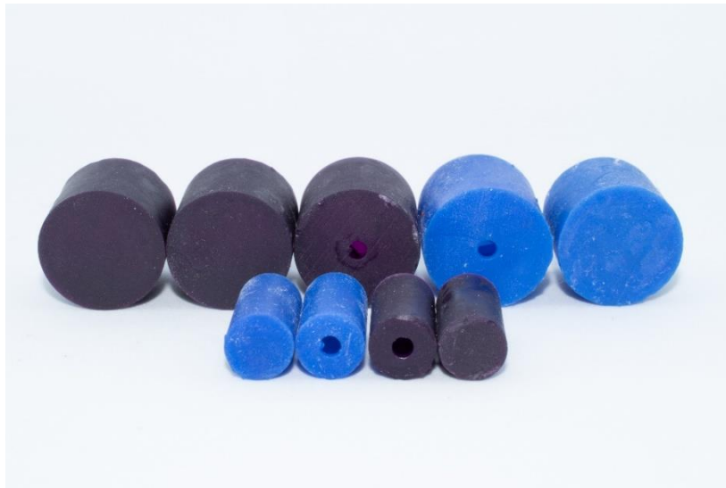
Fig.5. The figure illustrates all the types of the explored objects. The specimens made of Castable Wax ® are fabricated as: solid, hollow, hollow object with vents and two types depends on their size: type one – diameter – 20mm. and height – 20mm., type two – diameter – 10mm. and height 20mm. Identical specimens of Castable Resin ® are made.
