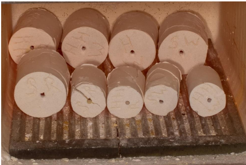
Fig.47. The experimental molds at 1050°C and after 60 min. hold.
