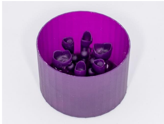
Fig.51. The object that is 3D printed consists of: a casting cone, a casting ring and a casting system, which are materialized as a single object.
