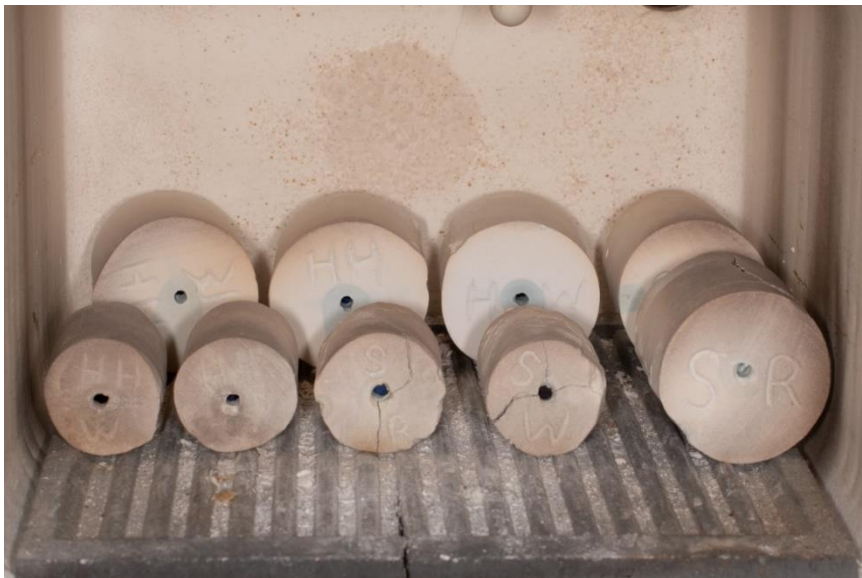
Fig.38. The fractures over the walls of the molds at 350°C.
