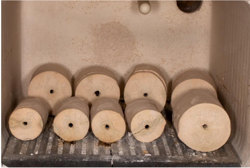
Fig.43. The observed molds after 30 min. hold at 250°C.
