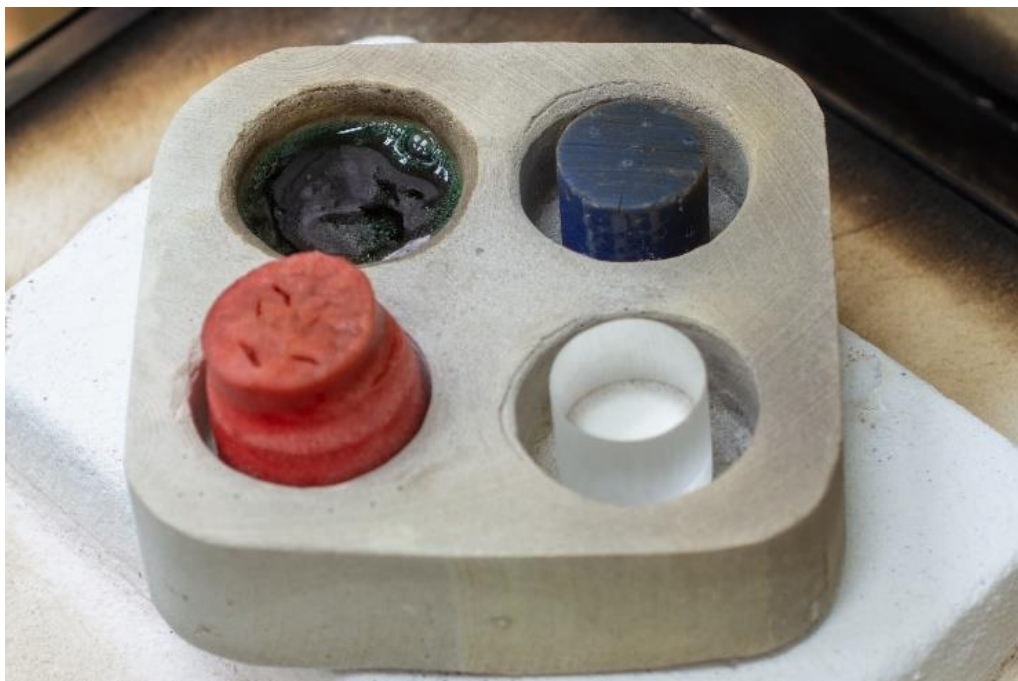
Fig.23. Structural changes of the samples at 300°C, after the 10 minutes hold.
