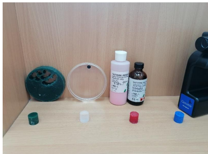
Fig.1. The examined samples are shown, from left to right as follows: CAD/CAM wax (Yeti Dental™), C-cast® (KaVo Dental™), Pattern resin LC® (GC™), and Castable Resin® (Formlabs™).
