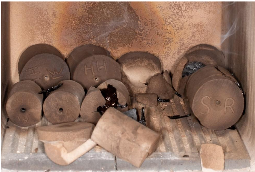
Fig.39. The results at 350°C. All of the mold are fractured, except these with hollow objects with vent invested.
