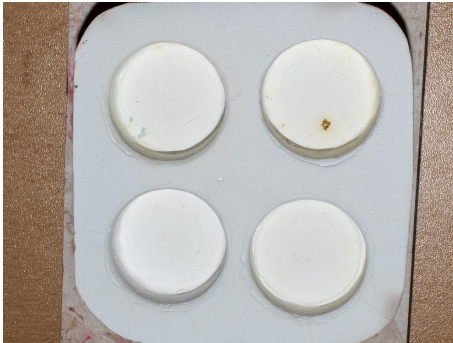
Fig.28. Residual ash amount reduction at 1050°C.
