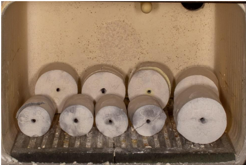
Fig.44. The experimental molds at 1050°C. There aren't any significant differences between this stage and 250°C as far as the mold surface is concerned.
