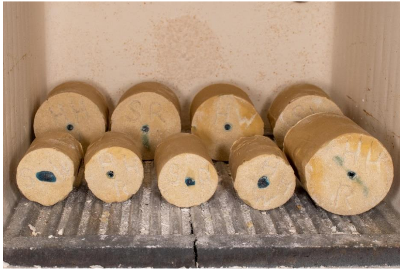
Fig.9. The observed molds made of WiroFine ® and inserted into the furnace at 25°C.
