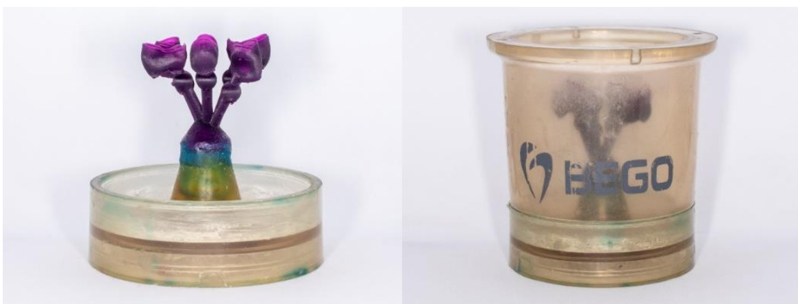
Fig.50. The sprue system is properly aligned and fixed to the casting cone.
