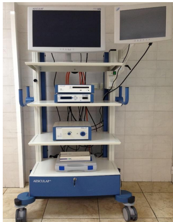
Fig. 1. Neuroendoscopic equipment: monitor, recording device, light source
